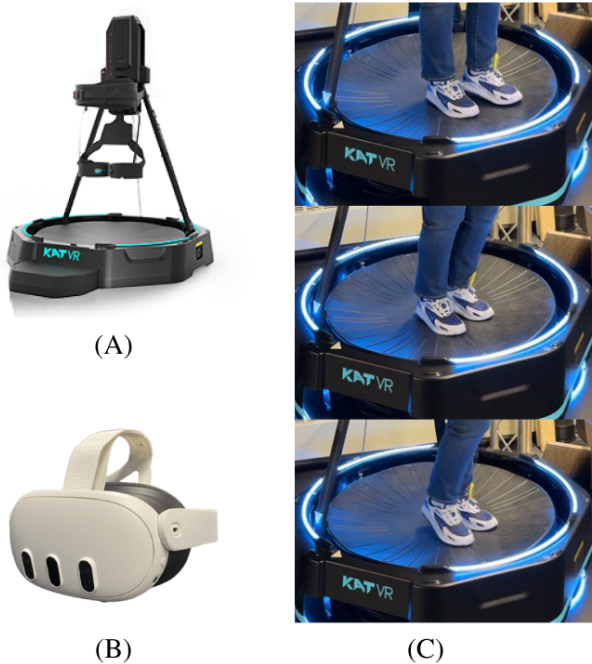
Figure 3: (A) Kat VR mini treadmill [31], (B) Meta Quest 3 VR Headset (C) Walking-in-place on the treadmill
